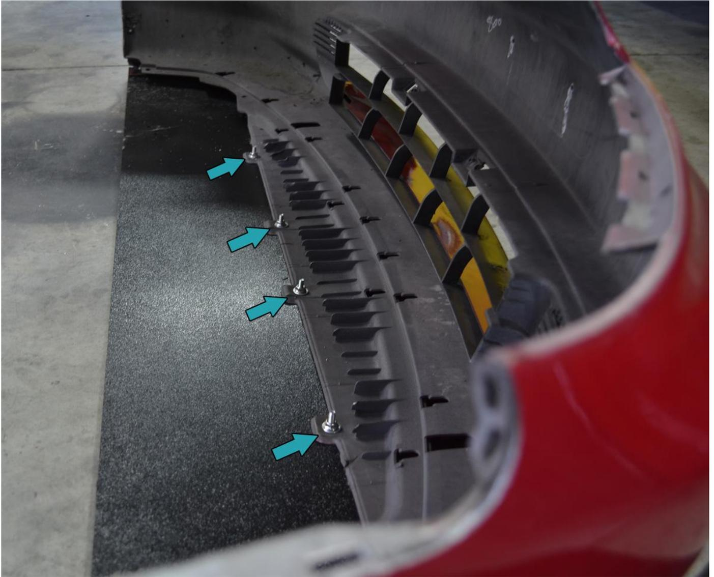
If your bumper has a lower slash guard we recommend using it for additional mounting points.
