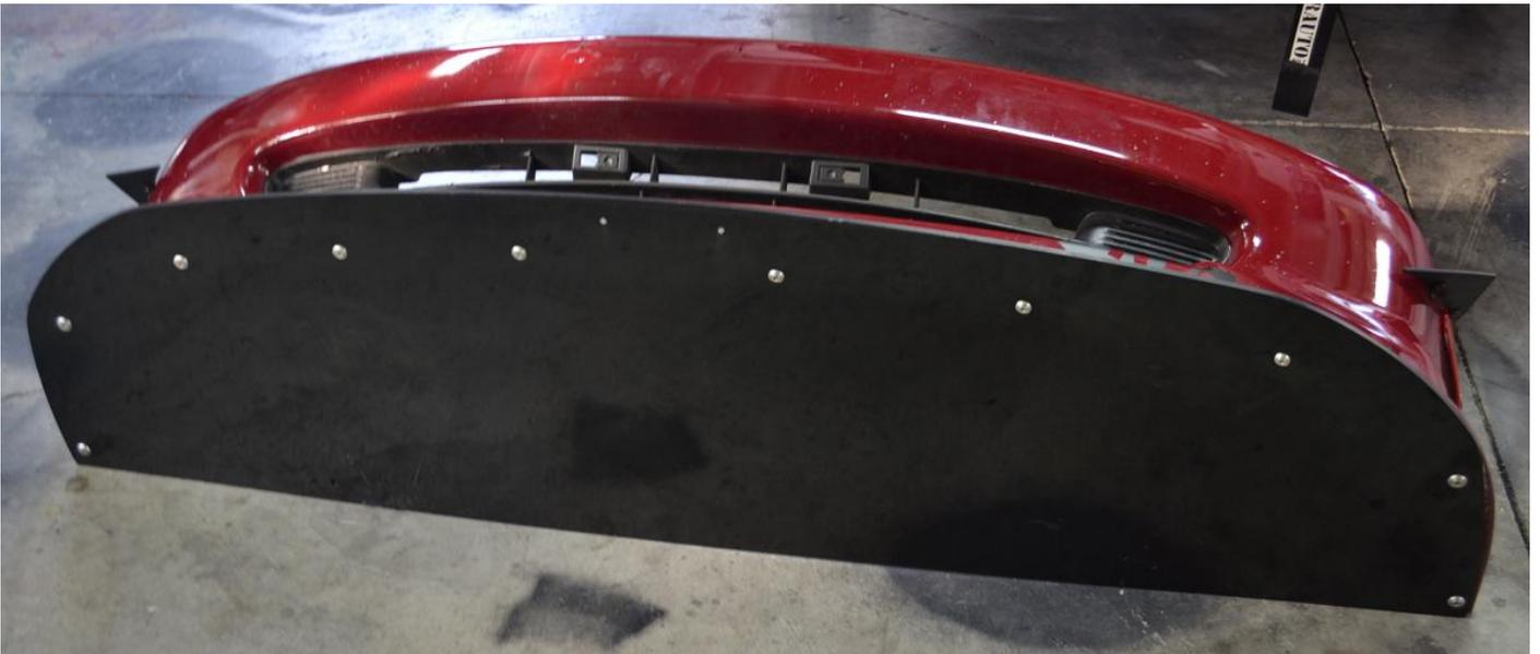
Mark and drill mounting points along the Splitter where you want it mounted to the bumper.
