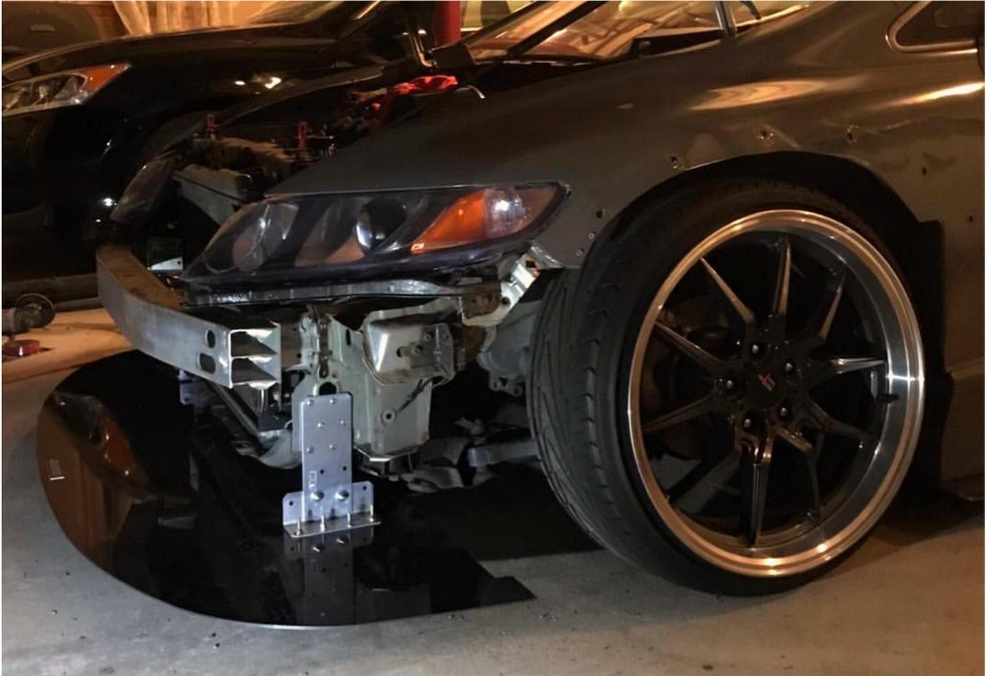
Custom brackets supporting the rear section of the Splitter via the radiator support.
