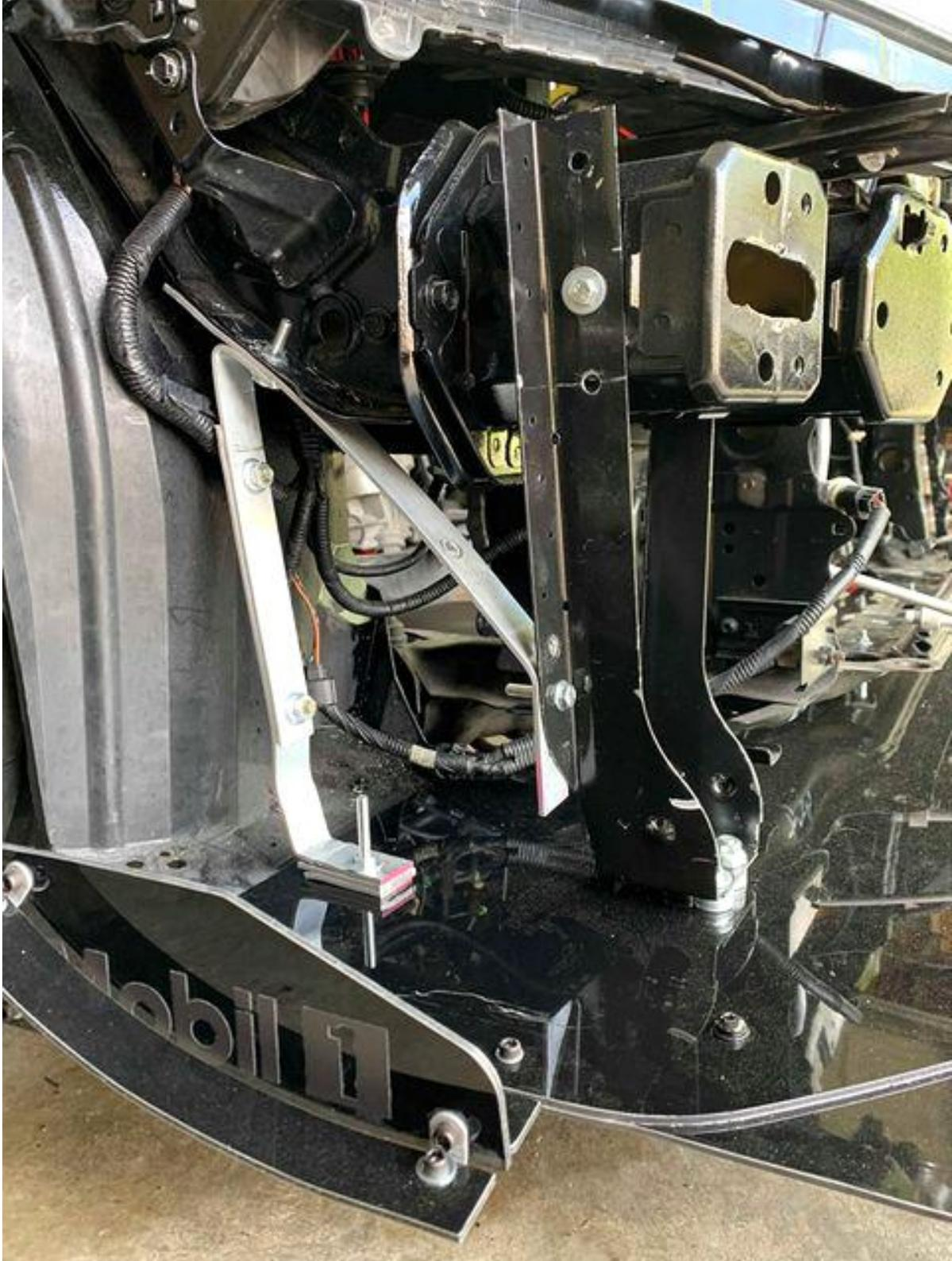
Custom brackets supporting the rear section of the Splitter via the bumper crash beam support rail.
