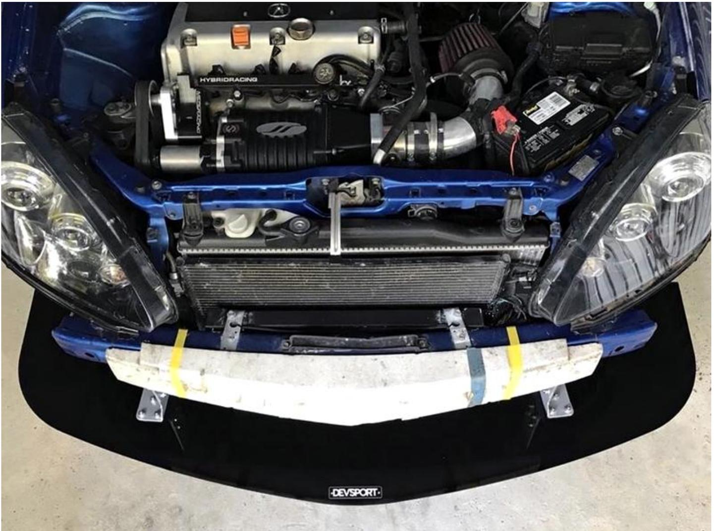
Once both brackets are installed, Lineup the Splitter and mark the holes for the Brackets. Drill the holes in the Splitter and mount the Splitter to the Brackets using the 5/16" x 7/8" bolts.
