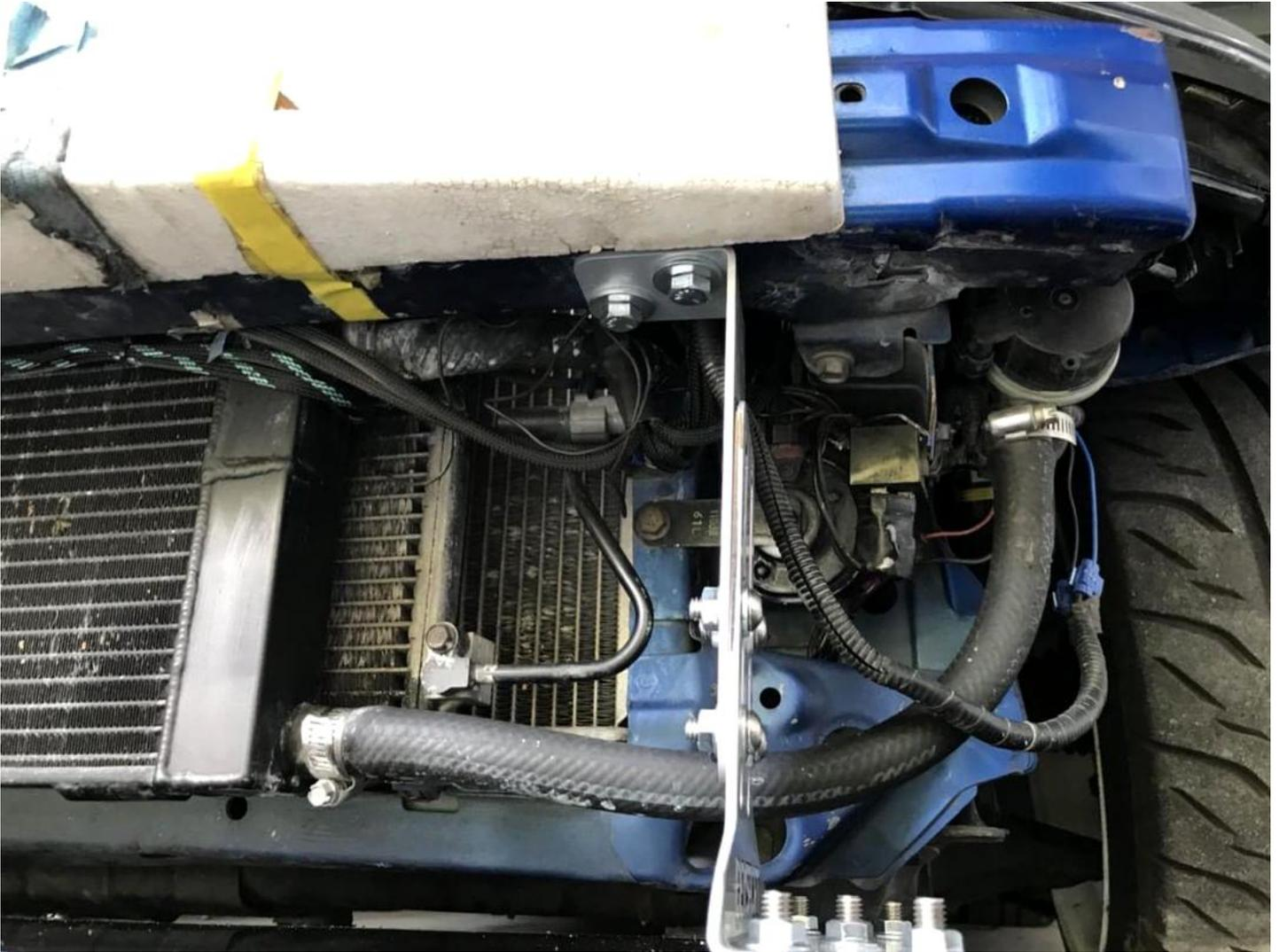
Place and mark the bolt holes of **Part B** (Upper Bracket) on the crash beam for each side.
