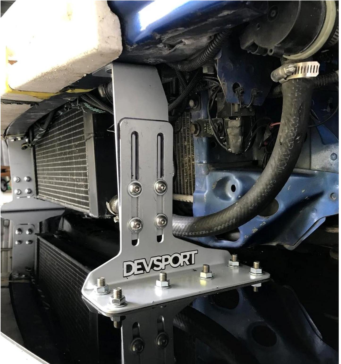
Bolt **Part A** (Lower Bracket) to **Part B** (Upper Bracket) using the 5/16" x 5/8" bolts. Leave the bolts a bit loose to adjust the height of the Brackets when installing the Front Splitter.
