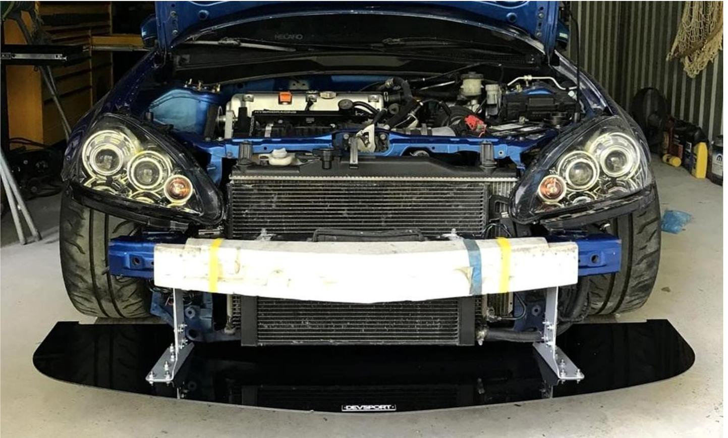
This picture references the approximate placement of the Brackets on the crash beam. The Brackets are to fit between the fog light and center grill of the bumper. **Refer to Step 5.**
